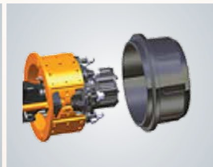
Biggest Brake Liners (325 mm x 155 mm) for Reduced Stopping Distance
