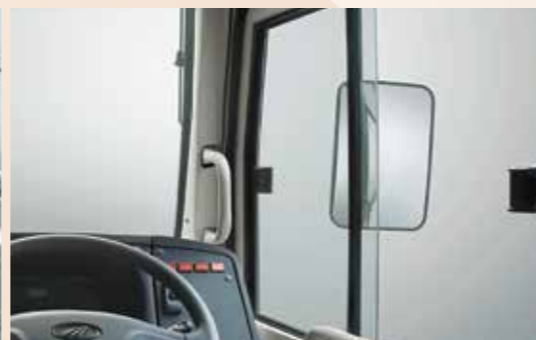
Wider Driver Door and Window as well as Foot Ventilation to Decrease Heat and Circulate Air Better for Driver
