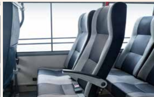
Ergonomically Designed Lumbar and Head Support. 295 mm Roomy Legroom. Wide Seat Pitch - 680 mm. Maximum Seat Depth - 415 mm
