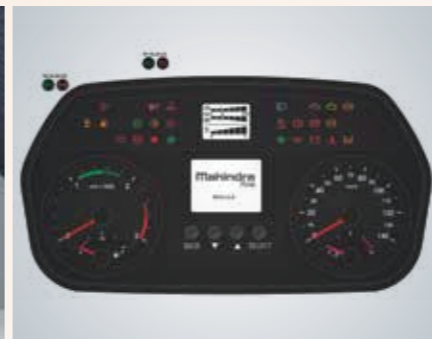
Driver-friendly Information System - Displays Average Mileage, Current Gear, Trip km and Air Pressure. Malfunction Indicators Help Prevent Breakdowns.
