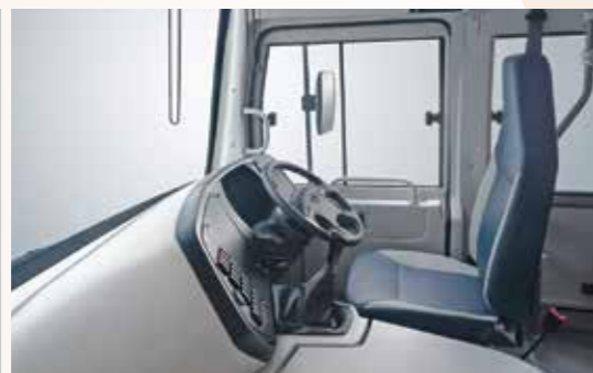
4-way Adjustable and Fully Reclining Driver's Seat
